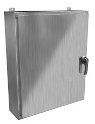
Hammond enclosure, NEMA 3R/4/4X/12/13, 36 x 30 x 8in (HxWxD), wall mount, 316 stainless steel, #4 brush finish, single-door, 3-point 316 stainless steel padlocking handle.
