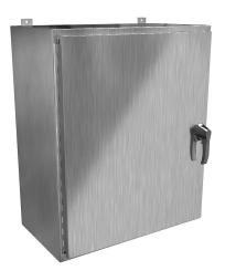
Hammond enclosure, NEMA 3R/4/4X/12/13, 36 x 30 x 16in (HxWxD), wall mount, 304 stainless steel, #4 brush finish, single-door, 3-point 316 stainless steel padlocking handle.
