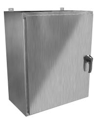
Hammond enclosure, NEMA 3R/4/4X/12/13, 36 x 30 x 16in (HxWxD), wall mount, 316 stainless steel, #4 brush finish, single-door, 3-point 316 stainless steel padlocking handle.
