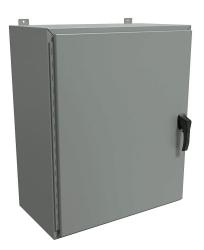
Hammond enclosure, NEMA 3R/4/12, 36 x 30 x 16in (HxWxD), wall mount, carbon steel, ANSI 61 gray, powder coat finish, single-door, 3-point padlocking handle.
