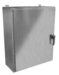
Hammond enclosure, NEMA 3R/4/4X/12/13, 36 x 30 x 12in (HxWxD), wall mount, 304 stainless steel, #4 brush finish, single-door, 3-point 316 stainless steel padlocking handle.
