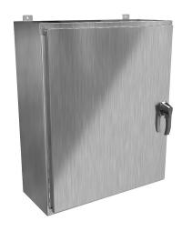
Hammond enclosure, NEMA 3R/4/4X/12/13, 36 x 30 x 12in (HxWxD), wall mount, 316 stainless steel, #4 brush finish, single-door, 3-point 316 stainless steel padlocking handle.
