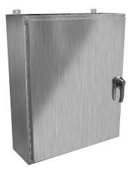
Hammond enclosure, NEMA 3R/4/4X/12/13, 36 x 30 x 10in (HxWxD), wall mount, 304 stainless steel, #4 brush finish, single-door, 3-point 316 stainless steel padlocking handle.
