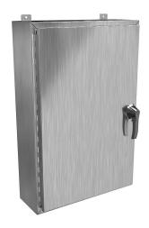
Hammond enclosure, NEMA 3R/4/4X/12/13, 36 x 24 x 8in (HxWxD), wall mount, 304 stainless steel, #4 brush finish, single-door, 3-point 316 stainless steel padlocking handle.
