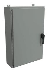
Hammond enclosure, NEMA 3R/4/12, 36 x 24 x 8in (HxWxD), wall mount, carbon steel, ANSI 61 gray, powder coat finish, single-door, 3-point padlocking handle.
