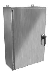
Hammond enclosure, NEMA 3R/4/4X/12/13, 36 x 24 x 10in (HxWxD), wall mount, 316 stainless steel, #4 brush finish, single-door, 3-point 316 stainless steel padlocking handle.
