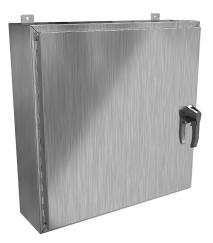
Hammond enclosure, NEMA 3R/4/4X/12/13, 30 x 30 x 8in (HxWxD), wall mount, 304 stainless steel, #4 brush finish, single-door, 3-point 316 stainless steel padlocking handle.
