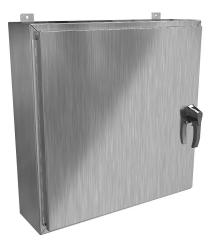
Hammond enclosure, NEMA 3R/4/4X/12/13, 30 x 30 x 8in (HxWxD), wall mount, 316 stainless steel, #4 brush finish, single-door, 3-point 316 stainless steel padlocking handle.
