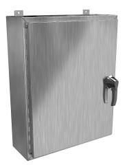
Hammond enclosure, NEMA 3R/4/4X/12/13, 30 x 24 x 8in (HxWxD), wall mount, 304 stainless steel, #4 brush finish, single-door, 3-point 316 stainless steel padlocking handle.
