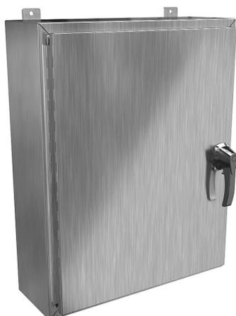
Hammond enclosure, NEMA 3R/4/4X/12/13, 30 x 24 x 8in (HxWxD), wall mount, 316 stainless steel, #4 brush finish, single-door, 3-point 316 stainless steel padlocking handle.
