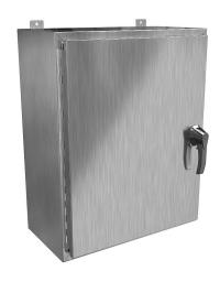
Hammond enclosure, NEMA 3R/4/4X/12/13, 30 x 24 x 12in (HxWxD), wall mount, 304 stainless steel, #4 brush finish, single-door, 3-point 316 stainless steel padlocking handle.
