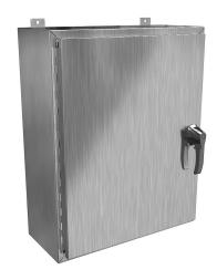
Hammond enclosure, NEMA 3R/4/4X/12/13, 30 x 24 x 10in (HxWxD), wall mount, 304 stainless steel, #4 brush finish, single-door, 3-point 316 stainless steel padlocking handle.
