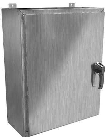
Hammond enclosure, NEMA 3R/4/4X/12/13, 30 x 24 x 10in (HxWxD), wall mount, 316 stainless steel, #4 brush finish, single-door, 3-point 316 stainless steel padlocking handle.
