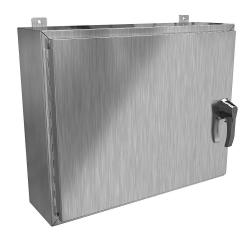
Hammond enclosure, NEMA 3R/4/4X/12/13, 24 x 30 x 8in (HxWxD), wall mount, 304 stainless steel, #4 brush finish, single-door, 3-point 316 stainless steel padlocking handle.
