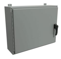
Hammond enclosure, NEMA 3R/4/12, 24 x 30 x 8in (HxWxD), wall mount, carbon steel, ANSI 61 gray, powder coat finish, single-door, 3-point padlocking handle.
