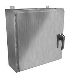
Hammond enclosure, NEMA 3R/4/4X/12/13, 24 x 24 x 8in (HxWxD), wall mount, 304 stainless steel, #4 brush finish, single-door, 3-point 316 stainless steel padlocking handle.
