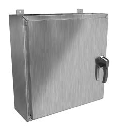
Hammond enclosure, NEMA 3R/4/4X/12/13, 24 x 24 x 8in (HxWxD), wall mount, 316 stainless steel, #4 brush finish, single-door, 3-point 316 stainless steel padlocking handle.
