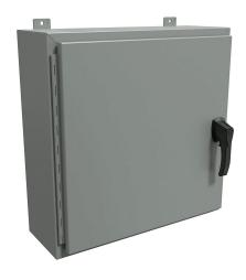
Hammond enclosure, NEMA 3R/4/12, 24 x 24 x 8in (HxWxD), wall mount, carbon steel, ANSI 61 gray, powder coat finish, single-door, 3-point padlocking handle.
