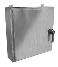
Hammond enclosure, NEMA 3R/4/4X/12/13, 24 x 24 x 6in (HxWxD), wall mount, 304 stainless steel, #4 brush finish, single-door, 3-point 316 stainless steel padlocking handle.
