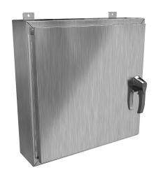
Hammond enclosure, NEMA 3R/4/4X/12/13, 24 x 24 x 6in (HxWxD), wall mount, 316 stainless steel, #4 brush finish, single-door, 3-point 316 stainless steel padlocking handle.
