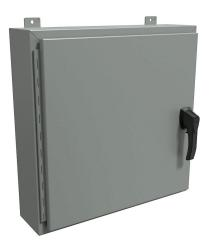
Hammond enclosure, NEMA 3R/4/12, 24 x 24 x 6in (HxWxD), wall mount, carbon steel, ANSI 61 gray, powder coat finish, single-door, 3-point padlocking handle.
