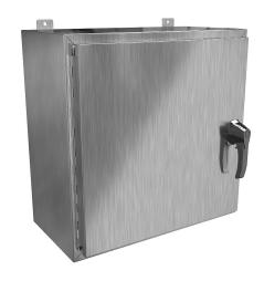
Hammond enclosure, NEMA 3R/4/4X/12/13, 24 x 24 x 12in (HxWxD), wall mount, 304 stainless steel, #4 brush finish, single-door, 3-point 316 stainless steel padlocking handle.
