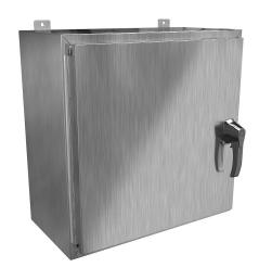
Hammond enclosure, NEMA 3R/4/4X/12/13, 24 x 24 x 12in (HxWxD), wall mount, 316 stainless steel, #4 brush finish, single-door, 3-point 316 stainless steel padlocking handle.
