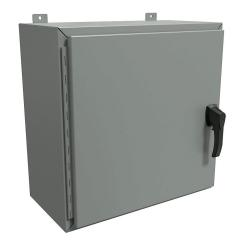
Hammond enclosure, NEMA 3R/4/12, 24 x 24 x 12in (HxWxD), wall mount, carbon steel, ANSI 61 gray, powder coat finish, single-door, 3-point padlocking handle.
