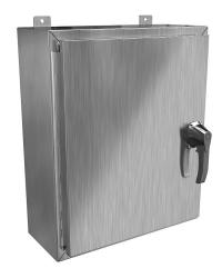
Hammond enclosure, NEMA 3R/4/4X/12/13, 24 x 20 x 8in (HxWxD), wall mount, 316 stainless steel, #4 brush finish, single-door, 3-point 316 stainless steel padlocking handle.
