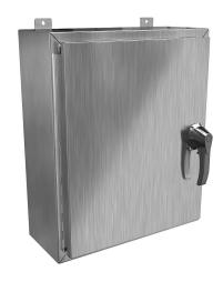
Hammond enclosure, NEMA 3R/4/4X/12/13, 24 x 20 x 8in (HxWxD), wall mount, 316 stainless steel, #4 brush finish, single-door, 3-point 316 stainless steel padlocking handle.
