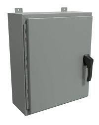
Hammond enclosure, NEMA 3R/4/12, 24 x 20 x 8in (HxWxD), wall mount, carbon steel, ANSI 61 gray, powder coat finish, single-door, 3-point padlocking handle.
