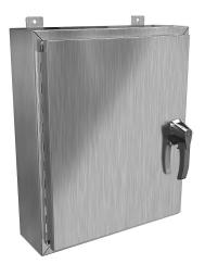
Hammond enclosure, NEMA 3R/4/4X/12/13, 24 x 20 x 6in (HxWxD), wall mount, 304 stainless steel, #4 brush finish, single-door, 3-point 316 stainless steel padlocking handle.
