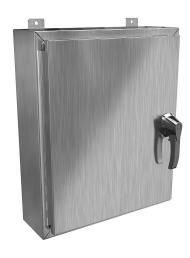
Hammond enclosure, NEMA 3R/4/4X/12/13, 24 x 20 x 6in (HxWxD), wall mount, 316 stainless steel, #4 brush finish, single-door, 3-point 316 stainless steel padlocking handle.
