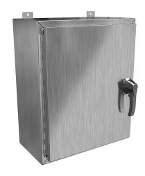
Hammond enclosure, NEMA 3R/4/4X/12/13, 24 x 20 x 10in (HxWxD), wall mount, 304 stainless steel, #4 brush finish, single-door, 3-point 316 stainless steel padlocking handle.
