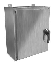
Hammond enclosure, NEMA 3R/4/4X/12/13, 24 x 20 x 10in (HxWxD), wall mount, 316 stainless steel, #4 brush finish, single-door, 3-point 316 stainless steel padlocking handle.
