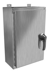
Hammond enclosure, NEMA 3R/4/4X/12/13, 24 x 16 x 8in (HxWxD), wall mount, 304 stainless steel, #4 brush finish, single-door, 3-point 316 stainless steel padlocking handle.
