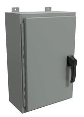
Hammond enclosure, NEMA 3R/4/12, 24 x 16 x 8in (HxWxD), wall mount, carbon steel, ANSI 61 gray, powder coat finish, single-door, 3-point padlocking handle.
