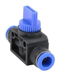
NITRA pneumatic push-to-connect fitting, union straight manual hand valve, 3-way, thermoplastic (PBT) body, (1) 5/16in (8mm) push-to-connect to (1) 5/16in (8mm) push-to-connect. Package of 2.
