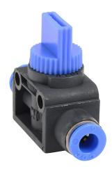
NITRA pneumatic push-to-connect fitting, union straight manual hand valve, 3-way, thermoplastic (PBT) body, (1) 6mm push-to-connect to (1) 6mm push-to-connect. Package of 2.
