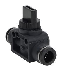
NITRA pneumatic push-to-connect fitting, union straight manual hand valve, 3-way, thermoplastic (PBT) body, (1) 5/16in (8mm) push-to-connect to (1) 5/16in (8mm) push-to-connect. Package of 2.
