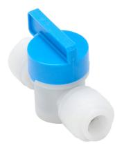
HydroMode potable water push-to-connect fitting, union straight manual hand valve, acetal body, (2) 5/16in tube connection(s), NSF/ANSI 61. Package of 2.
