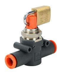
NITRA pneumatic push-to-connect fitting, inline manual shutoff valve, locking, 3-way, technopolymer body, (1) 5/16in (8mm) push-to-connect to (1) 5/16in (8mm) push-to-connect.
