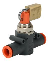
NITRA pneumatic push-to-connect fitting, inline manual shutoff valve, locking, 2-way, technopolymer body, (1) 5/16in (8mm) push-to-connect to (1) 5/16in (8mm) push-to-connect.
