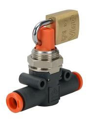
NITRA pneumatic push-to-connect fitting, inline manual shutoff valve, locking, 3-way, technopolymer body, (1) 1/4in push-to-connect to (1) 1/4in push-to-connect.
