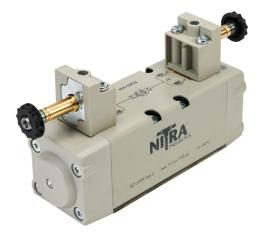
NITRA solenoid valve, ISO 5599/1 size 2, 5-way, 3-position, center pressure, double solenoid, aluminum alloy body, locking manual override.
