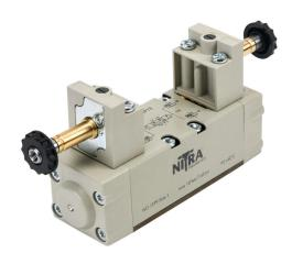
NITRA solenoid valve, ISO 5599/1 size 1, 5-way, 3-position, center pressure, double solenoid, aluminum alloy body, locking manual override.
