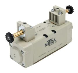
NITRA solenoid valve, ISO 5599/1 size 2, 5-way, 3-position, center exhaust, double solenoid, aluminum alloy body, locking manual override.
