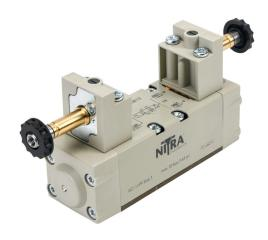
NITRA solenoid valve, ISO 5599/1 size 1, 5-way, 3-position, center exhaust, double solenoid, aluminum alloy body, locking manual override.
