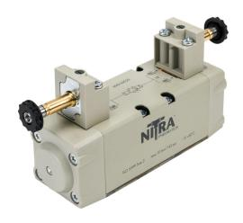
NITRA solenoid valve, ISO 5599/1 size 2, 5-way, 3-position, center closed, double solenoid, aluminum alloy body, locking manual override.
