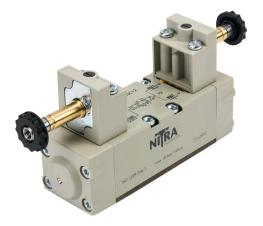
NITRA solenoid valve, ISO 5599/1 size 1, 5-way, 3-position, center closed, double solenoid, aluminum alloy body, locking manual override.
