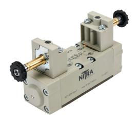
NITRA solenoid valve, ISO 5599/1 size 1, 5-way, 3-position, center closed, double solenoid, aluminum alloy body, locking manual override.
