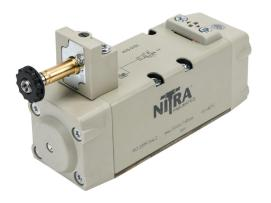
NITRA solenoid valve, ISO 5599/1 size 2, 5-way, 2-position, single solenoid spring return, aluminum alloy body, locking manual override.
